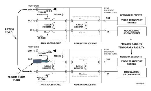
Figure 33. Temporary Same Video Signal Distribution to Second Location
